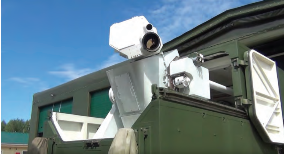
The Trailer-Mounted Peresvet Laser Weapon System. Some observers suspect that the laser's power levels will allow it to target satellites in LEO.
